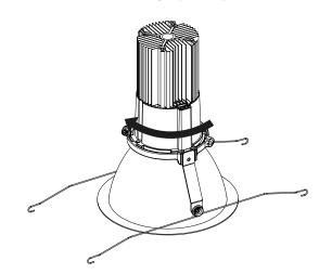
3 Attach the ground wire terminal (factory installed) to the housing using an existing screw inside the housing.
