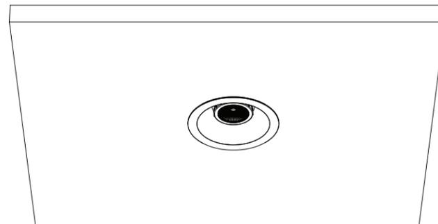
**8** To adjust, rotate and tilt light module to direct light until desired lighting coverage is achieved.
