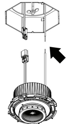
**3** Connect module female connector to hardwire adapter male connector.
