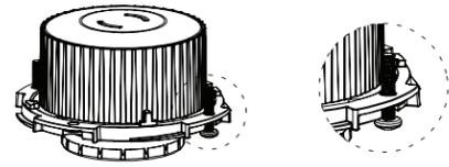
**5** Carefully route wires into junction box and place module into junction box, aligning screws to screw holes in junction box bracket. Screw to junction box.
