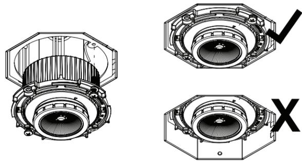
**6** Align trim onto module and turn trim clockwise until secure.
