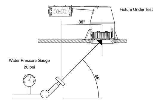
The test is performed over four hours and is sequenced as follows,
