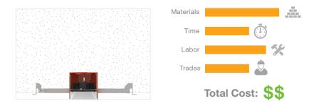
The OneFrame<sup>™</sup> junction box reduces installation costs significantly because it eliminates the requirement to create boxed-out cavities at the time of construction by utilizing one of the exceptions provided by subsection 714.5.2:
