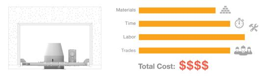
Although this is an effective method, it requires the ceiling space to have boxed-out cavities, using the same fire-rated membrane material, to mount the recessed fixtures in. This approach adds significant costs and requires extra space above the ceiling plane that may not always be available.
