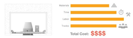
Although this is an effective method, it requires the ceiling space to have boxed-out cavities, using the same fire-resistance rated membrane material, to mount the recessed fixtures in. This approach adds significant costs and requires extra space above the ceiling plane that may not always be available.
